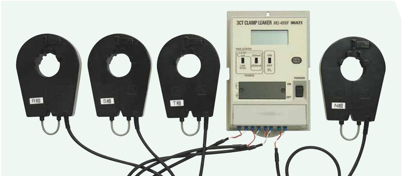
New Method-Can Measure Leakage Current by clamping 3 or 4 CTs respectively to the conductors
