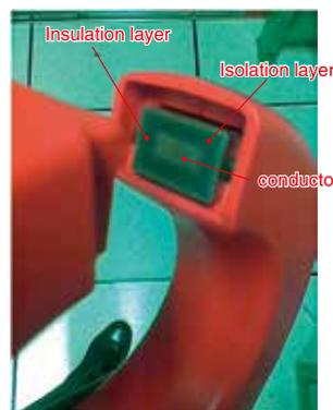
Plane clamp head is easily to become dirty. Magnetic can not coherent with single isolation layer easily.
